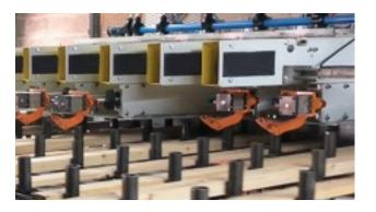
This system uses the optimiser's solutions to accurately position lumber boards prior to trimming operation at the green or dry mill.
