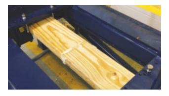
This system has been specially developed to control the quality of finger joint wood connections.
