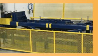
The TNS-800 tensile test bench will meet your load capacity requirements for TESTING EITHER YOUR ENGINEERED BUILDING COMPONENTS OR LUMBER SPECIALITIES
